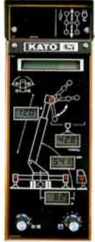
tection in the unlikely event of a malfunction in the ACS Moment Limiter or any other problems, a trouble indicator has been provided to generate an emergency signal in the appropriate display to warn the operator.
